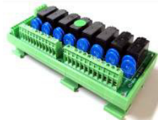
M4901 8 voltage free relay outputs rated to 250VAC 8A
