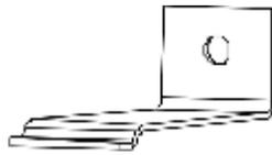
The unit is installed using four stainless steel mounting brackets, which slot into the front slots in the top and bottom of the case. The figure below shows the way in which the clip fits into the case slot. Two clips are required on both top and bottom. The hole in each clip is 7mm in diameter.
