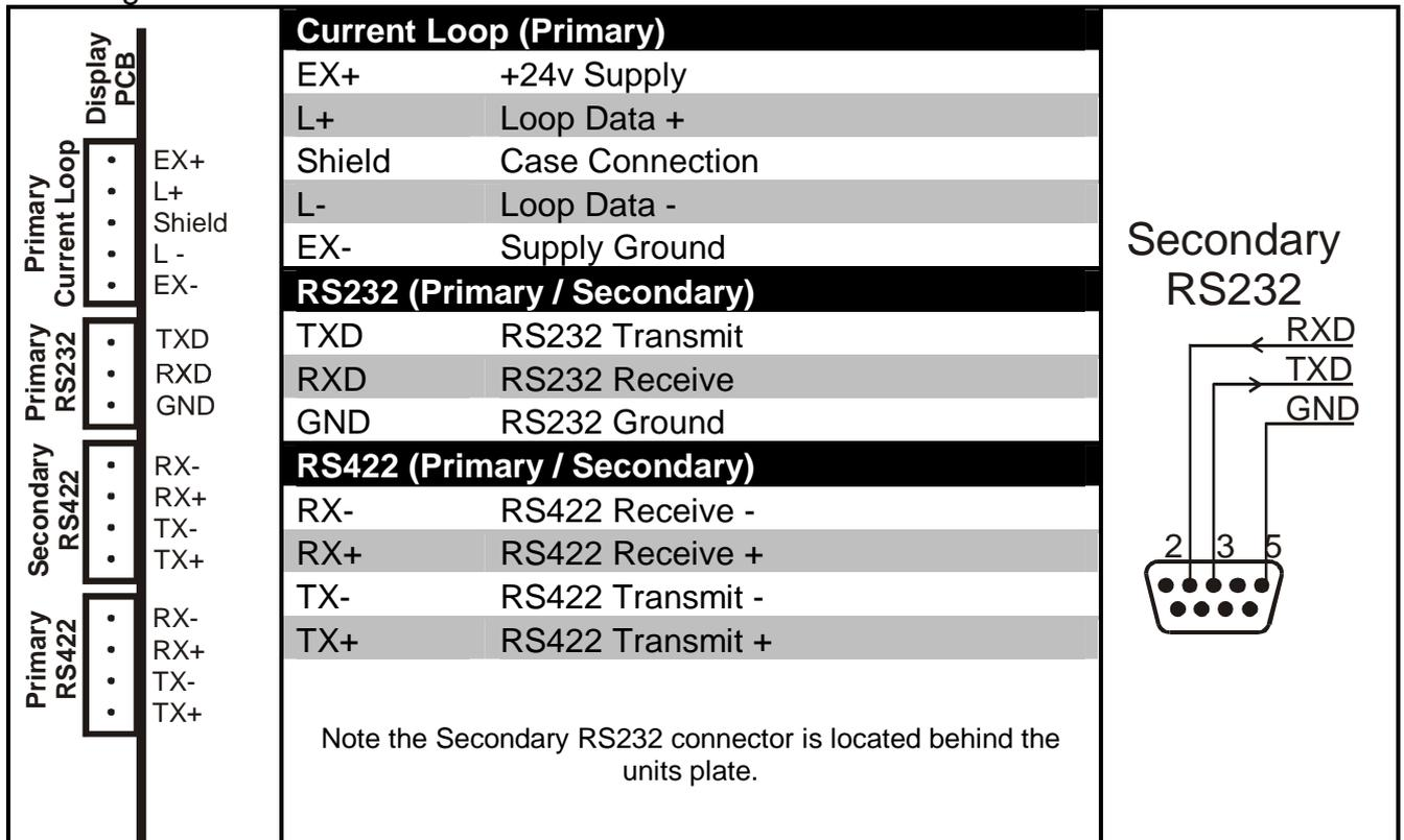
The serial connection to the **6500** provides the source of data. A shielded data cable should be used to prevent electrical noise interfering with the signal on the cable, and thereby the operation of the unit. Note that RS232 is not suitable for long cable runs or electrically noisy environments.
