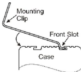
When disengaging a clip maintain tension to draw the clip towards the back of the case, as shown in the figure at left. This will ensure that a clearance is maintained and the clip can move more easily in the slot.
