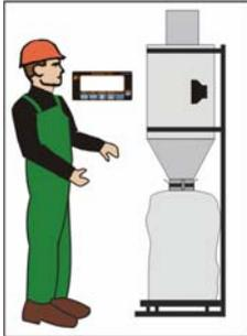
A weighing machine is to be used in a single-speed, single material, bag/box filling application using a 2100. The 2100's in-flight compensation automatically adjusts the in-flight value at the end of every batch. The 2100 can alert the operator to manually remove the filled bag/box or it can trigger an external mechanism to remove the filled bag/box. For 2100 - Bag Filler Using a Two-Speed Feeder refer to Application Note 3.
