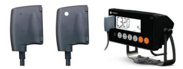
The rinLINK provides an isolated optical serial connection directly to the front of the indicator. It is magnetically coupled for easy access on site for updates/ setup of the indicator. The rinLINK can be used to download new firmware or provide the connection to the PC running Viewer for indicator configuration.
