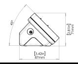
C320-H with Fully Sealed Boot, Plug Pack and Stainless Steel Bracket
