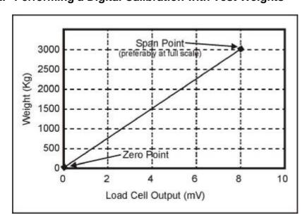
Figure 30: Chart - Zero and Span Points to Interpolate Weight from Load Cell
