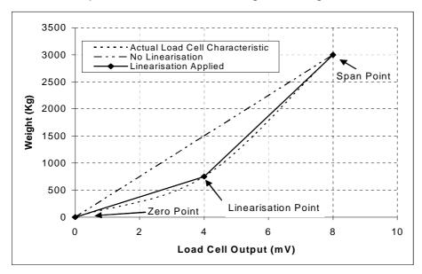
Figure 31: Chart - Non-Linear Characteristic for Load Cell Output
