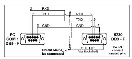
Figure 7: RS-232 - Networking Connection
