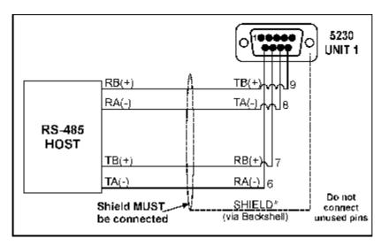
Figure 8: RS-485 – Networking Connection
