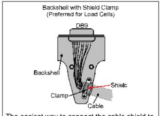
The easiest way to connect the cable shield to the DB9 backshell is to fold the shield wires back over the outside of the cable insulation so the cable clamp of the backshell makes good electrical contact with the shield when installed.
