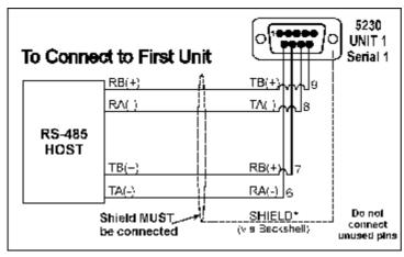
Figure 9: Multi-Drop Networking Connections - Connecting to First Unit
