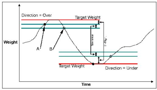
Figure 32: Setpoint Operation – Over vs Under
