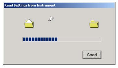
• After the settings have been read completely the **5230 Viewer** will reflect the actual display on the instrument as well as showing extra Tabs for changing settings.
