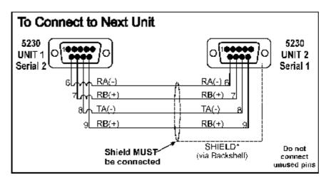
Figure 10: Multi-Drop Networking Connections - Connecting to Next Unit
