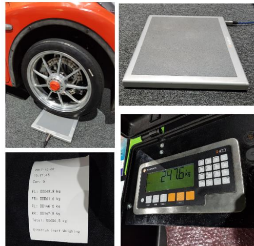
Clockwise from Top Left: Car being weighed, load cell close-up, R423 indicator, print-out of car weight
