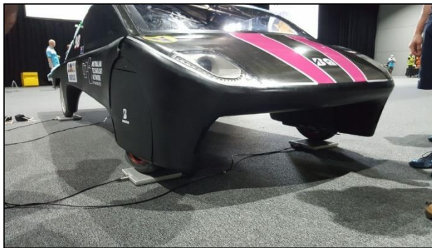
Vehicle weight and balance being measured
