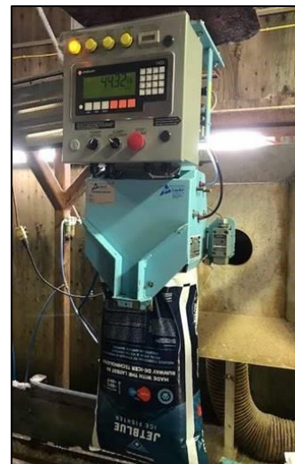
The panel mounted R423 Indicator used in the packing system.
