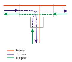
2.3. Various network configurations can be created using a combination of Tjunctions:
