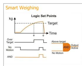
R400 Logic set points are based on the status of the inputs and the defined mask that is used to match IO1-IO24 for the logic set points.
