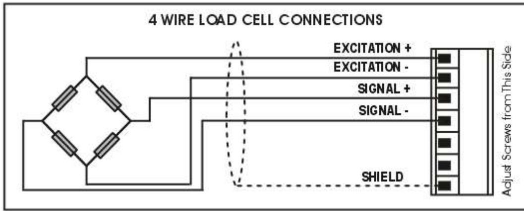
Figure 3: 4-Wire Connections
