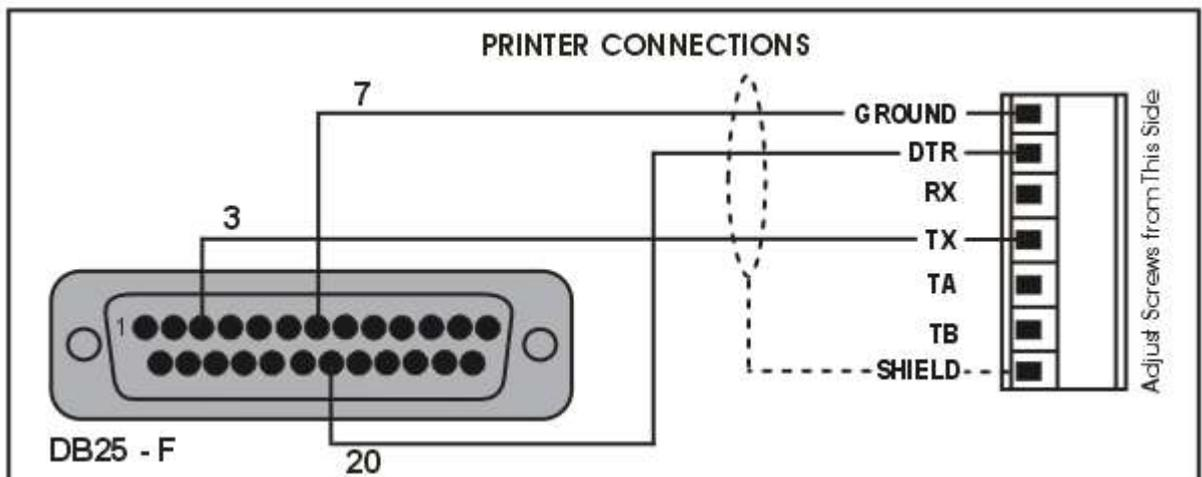
Figure 6: RS-232 – Instrument to Printer (DB25)
