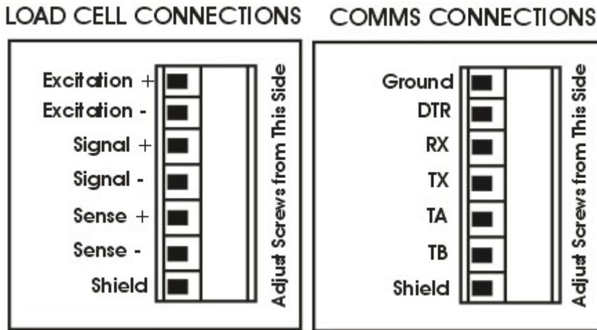
Figure 2: Cable Connections
