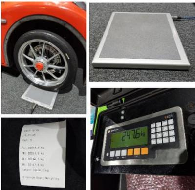
*Rinstrum Instruments at work – Loadcell, Indicator and Print-out*
